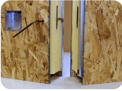
(photo shows cam-wrench, cam-locks, tongue-and-groove panel connection system with metal splines, polyurethane foam core and OSB substrates)
